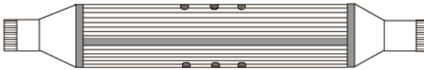
Fig. 1-5 Comparison of interchangeable loading sections of Serata Probe for choice of high-accuracy stress measurement by single-fracture method or faster property measurement by double-fracture method
